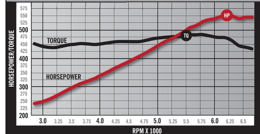
**HP** PEAK HORSEPOWER: 552 @ 6,200 **TQ** PEAK TORQUE: 484 FT.-LBS. @ 5,500
